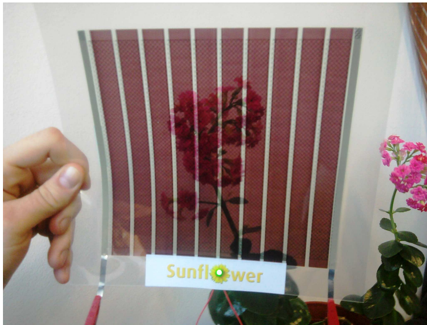
Figure 2: Konarka OPV demonstrator operates an LED in indoor conditions
