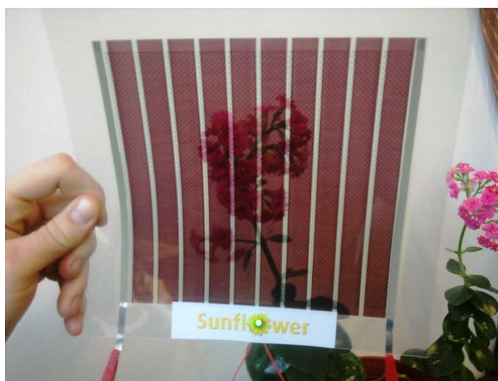
Figure 3: Konarka OPV demonstrator operates an LED in indoor conditions
